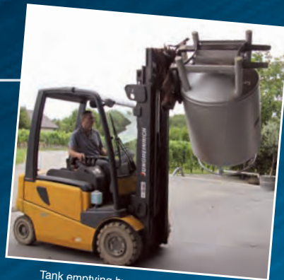
Tank emptying by means of rotating jig
