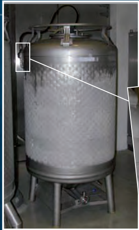
Jacketed for cooling to -5^{\circ}\text{C}
