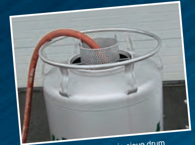
Discharge of juice via sieve drum
