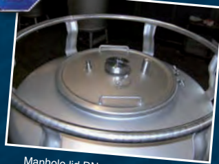
Manhole lid DN 400 (16") with gas inlet valve and pressure relief valve
