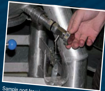
Sample port for wine tasting, via quick coupling
